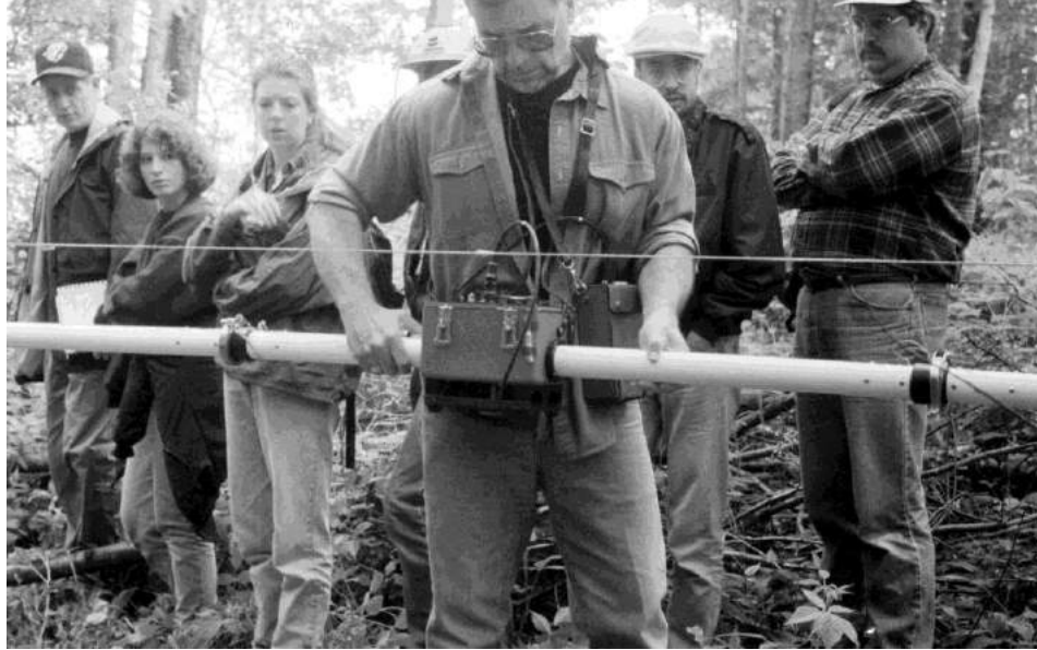
An EM Ground Conductivity Meter being used to locate sub-surface anomalies as an electromagnetic induction (EMI) technique
