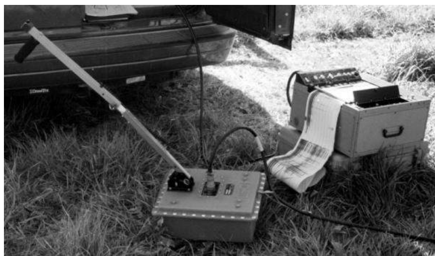
Older model of ground penetrating radar equipment used in search for clandestine grave
